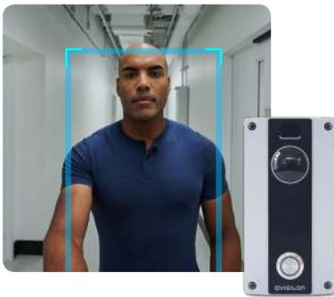
Using ACM<sup>TM</sup> and ACC<sup>TM</sup> software, you can instantly verify if a person seen carding in on camera matches the ID photo associated with the access card they're using, then lock or unlock the door right from your ACC dashboard.
